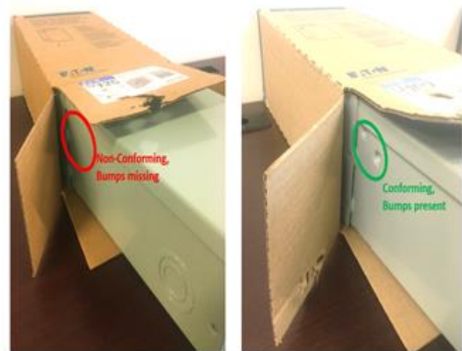
Figure 2 – Product being pulled out of cartons. Red circle shows missing bumps on the case. Green circle shows conforming product with visible bumps.
