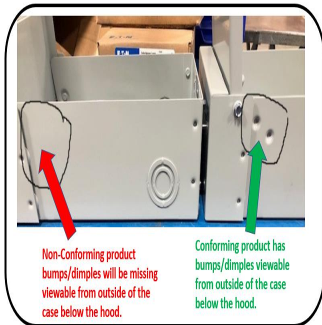
Figure 3 – (Red) -Case on the left defective with missing inner cover support bumps. (Green) Case on the right with inner cover bumps.
