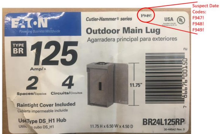
Figure 1 – Typical Carton Label & Date Code location. “F9” Indicates Year 2019 and “49!” indicates 49 th week of production. Affected product are from weeks 47, 48, 49
